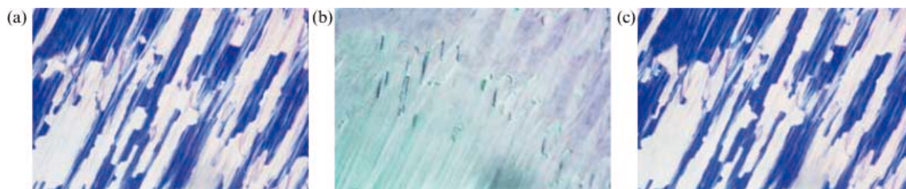
Figure 6. Field effect on the SmC phase of 4r-8 at 155.0°C in a cell of 5 \mu\text{m} thickness treated for parallel alignment. The alignment direction is rotated by 15^\circ . The applied sc field was (a) 2.6, (b) 0 and (c) -2.6 \text{ V } \mu\text{m}^{-1} . The horizontal edge is 0.75 mm.
